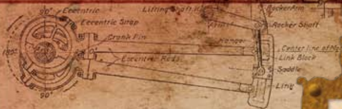
Fig. 64. Standard Stephenson Valve Gear.
