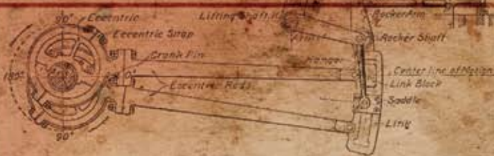
Fig. 64. Standard Stephenson Valve Gear.
