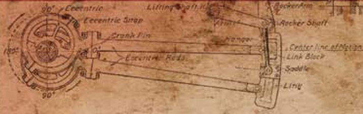
Fig. 64. Standard Stephenson Valve Gear.
