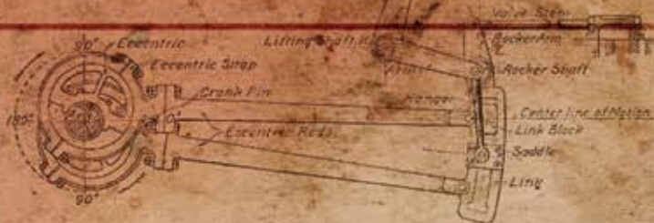
Fig. 64. Standard Stephenson Valve Gear.
