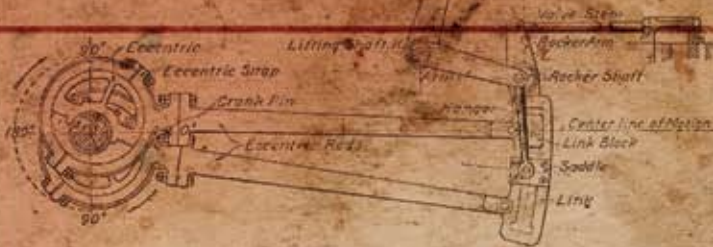
Fig. 64. Standard Stephenson Valve Gear.
